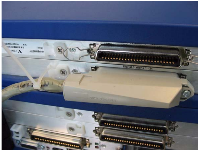
Figure 4-3 Connecting a cable to an RJ-21X connector—90° method
